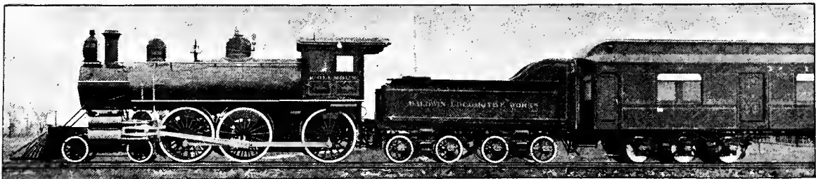
Fig. 2423. Side View. THE PULLMAN VESTIBULE FOR A LOCOMOTIVE TENDER. (Exhibited at the World's Columbian Exposition, 1893, but not in general use.)
